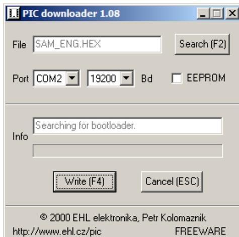
Press the reset button on the SAM-III controller PCB. The PIC downloader should immediately start writing the file as shown below. If there is no response, momentarily disconnect the power from the SAM-III to force a hard reboot. The PIC downloader should starting writing.
