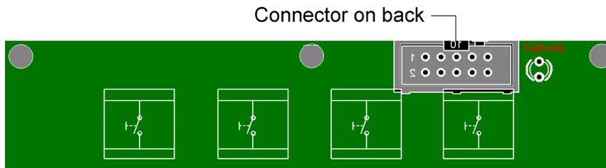
Install the four pushbuttons and red LED on the top (silkscreen side) and the ribbon cable socket on the bottom:
