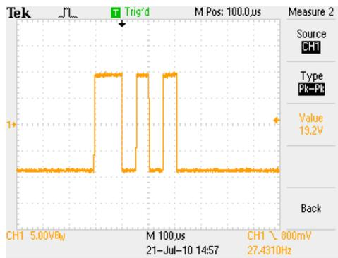
SAM-III → PC, measured at Pin 3 of JP1 while waiting to press RESET to download IB3\_ENG.HEX:
