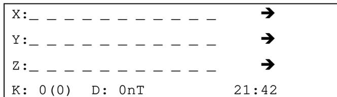
The display indicates blank magnetic induction values. Actual values will not be displayed until sensors are connected. The next section describes the display layout for reference purposes.
