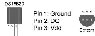
**Note:** Because the 1-wire bus protocol was not designed for distance, the temperature sensor cannot be located more than approximately 2 m from the SAM-III processor module. This precludes collocating the temperature sensor with the magnetometer sensors where the magnetometer sensors are remotely located (which will be the case in almost all applications).
