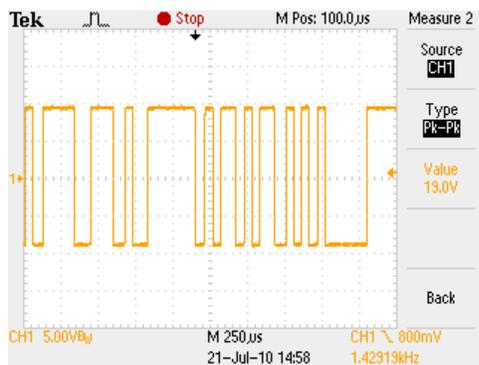
PC → SAM-III, measured at Pin 2 of JP1 after pressing RESET and while receiving IB3\_ENG.HEX from PIC
