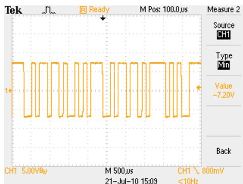
SAM-III → PC, measured at Pin 3 of JP1 while sending sensor data text to HyperTerminal: Image
