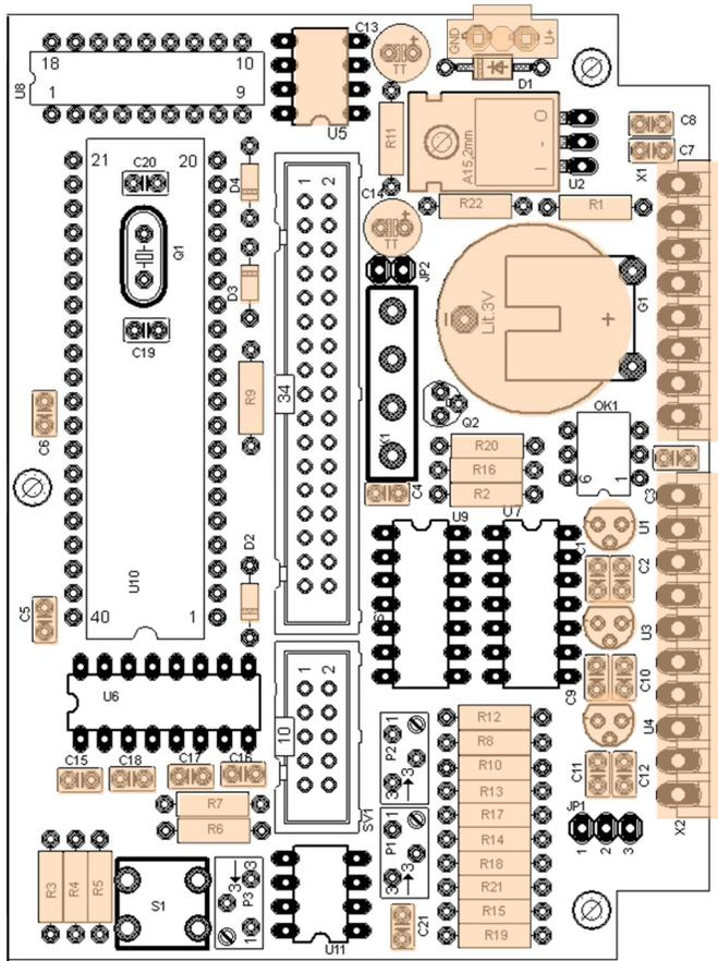
Install all listed components on the top (silkscreen) side of the PCB and solder at the bottom. A larger image of the PCB is shown in Sect. XIX.
