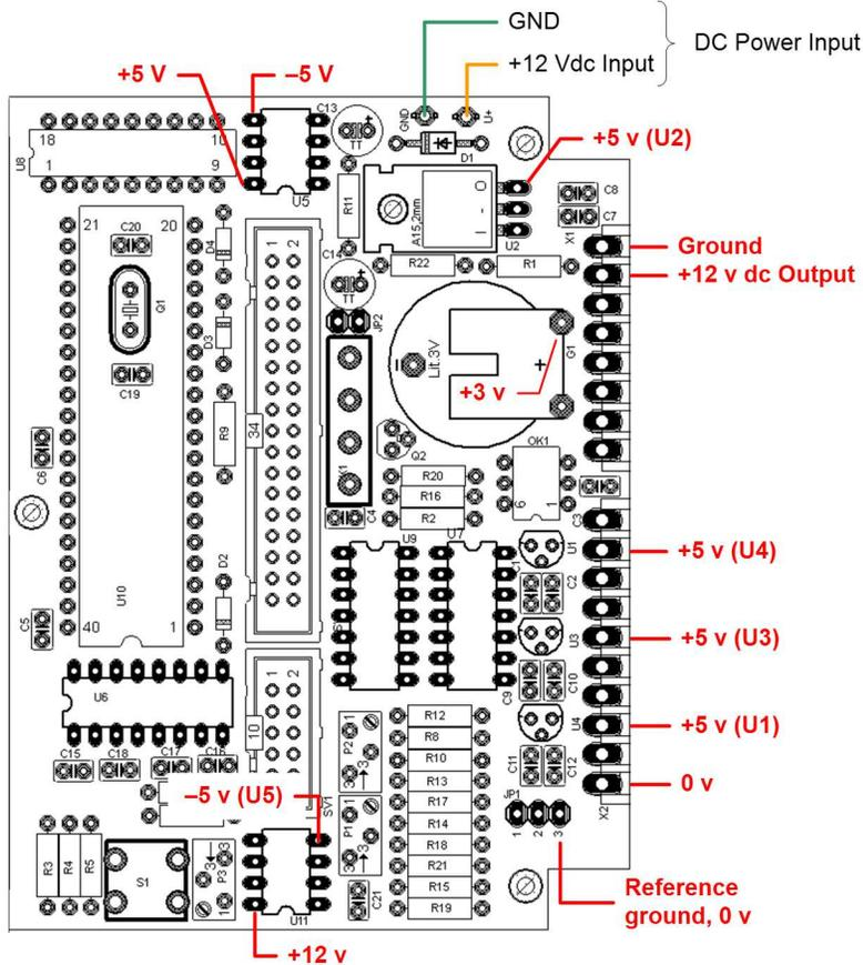
If all voltages are within the specified ranges, the power supply components are working properly. Remove the dc power before continuing!
