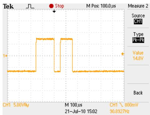
SAM-III  $\rightarrow$  PC, measured at Pin 3 of JP1 while sending "RS232" text to HyperTerminal: Image F0005TEK
