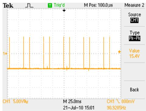
SAM-III  $\rightarrow$  PC, measured at Pin 3 of JP1 while downloading IB3\_ENG.HEX from PIC downloader: Image F0004TEK (different timebase than F0003TEK)
