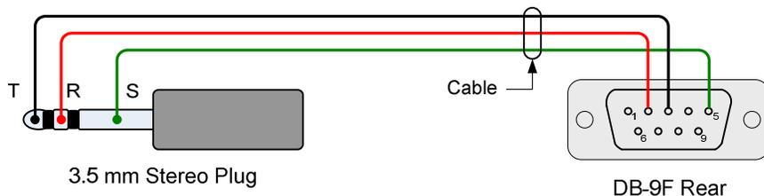
Some data loggers (for example, the Onset Computer HOBO and Omega Engineering data loggers) use the same configuration, so users with these data loggers already have a cable and do not need to make one.
