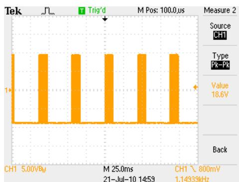
SAM-III → PC, measured at Pin 3 of JP1 after pressing RESET and while downloading IB3\_ENG.HEX from
