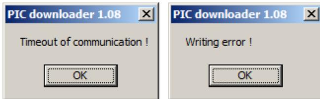
there was a communication problem with the serial port. Sometimes this can be resolved by unplugging and then plugging the USB connector on the USB-serial adapter. If that does not work, use PortMon to analyze the serial connection (see appendix). See also oscilloscope screenshots below as a troubleshooting aid if you have an oscilloscope.
