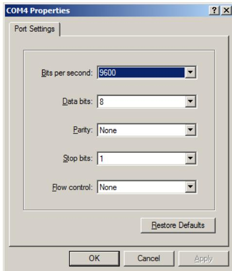
Adjust the settings in the drop-down boxes as follows: 9600 Bits per second – 8 Data bits – Parity None – Stop bits 1 – Flow control None. Click OK. If necessary, press the Call icon button on the HyperTerminal menu bar.
