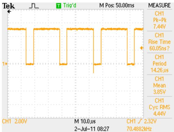
The three scope images show, in order, U10 pin 16 and 18 (programmable outputs RC1 and RC3 to multiplexer) and pin 15 (programmable input RC0 from sensors)
