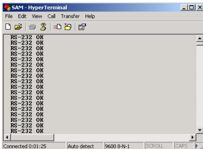
If nothing happens, try unplugging the USB connector of the USB-serial adapter and plugging it back into the PC. There is considerable variability in USB-serial adapters leading to many problems with serial port testing.
