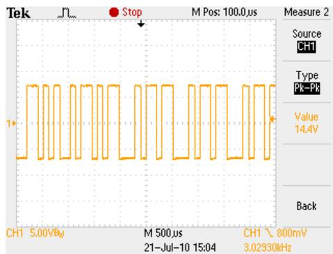
PC  $\rightarrow$  SAM-III, measured at Pin 2 of JP1 while sending "RS232" text to HyperTerminal: Approximately  $-9$  Vdc
