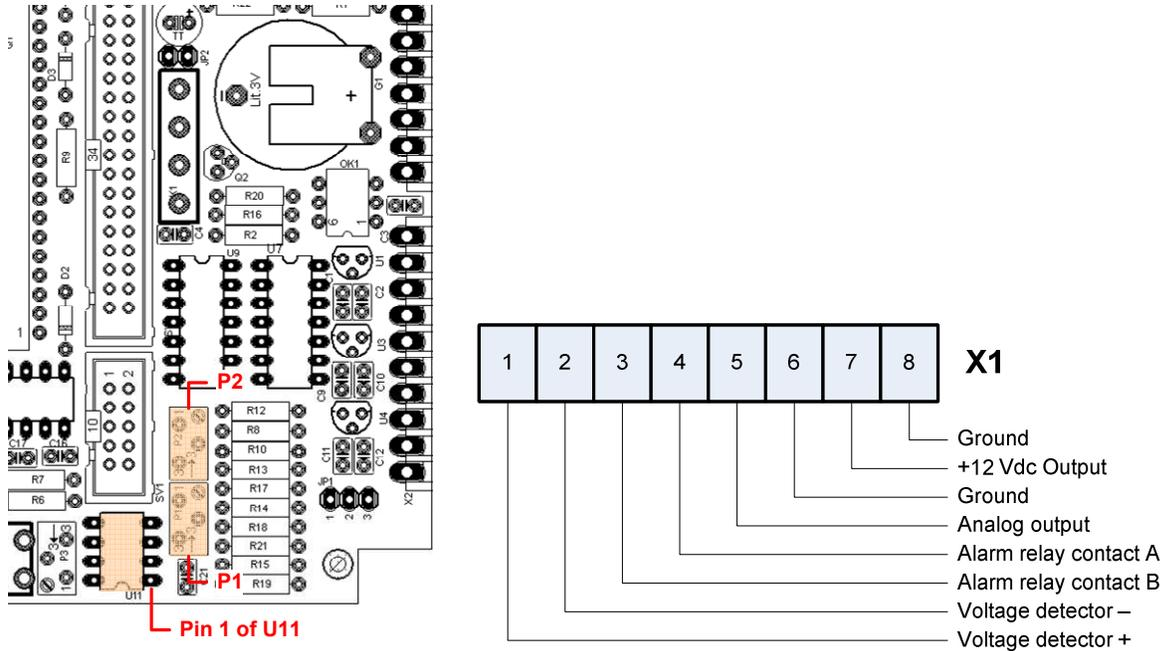
Set the multimeter to the 20 Vdc range, and connect the meter negative lead to position 6 (ground) of X1.
