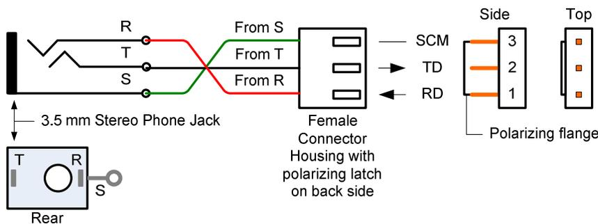
Of course, a cable with DB-9 connectors at each end will not work with this arrangement for connecting the SAM-III to a PC, but an existing cable with at least one DB-9F connector can be easily modified. Cut off one of the connectors (retain one DB-9F on the cable) and wire the cable blunt end to a 3.5 mm stereo plug as shown in the drawing below.
