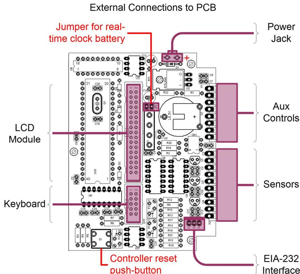
Install the shorting block on JP2 to activate the internal real time clock battery
