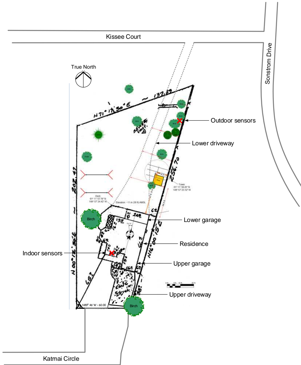
Figure 3 ~ Plat showing SAM-III sensor locations and other details. The permanently buried outdoor sensor fixture is indicated by the red X at upper-right of the trapezoidal property. The temporary indoor fixture is indicated by the red X at lower-middle of the plat, inside the residence. Property lines are thick black lines, and roads and driveways are thick gray lines. For reference, the eastern property line is 78.2 m (256.7 ft). Katmai Circle, Sonstrom Drive and Kissee Court are not built for through traffic and serve only a few local residences.
