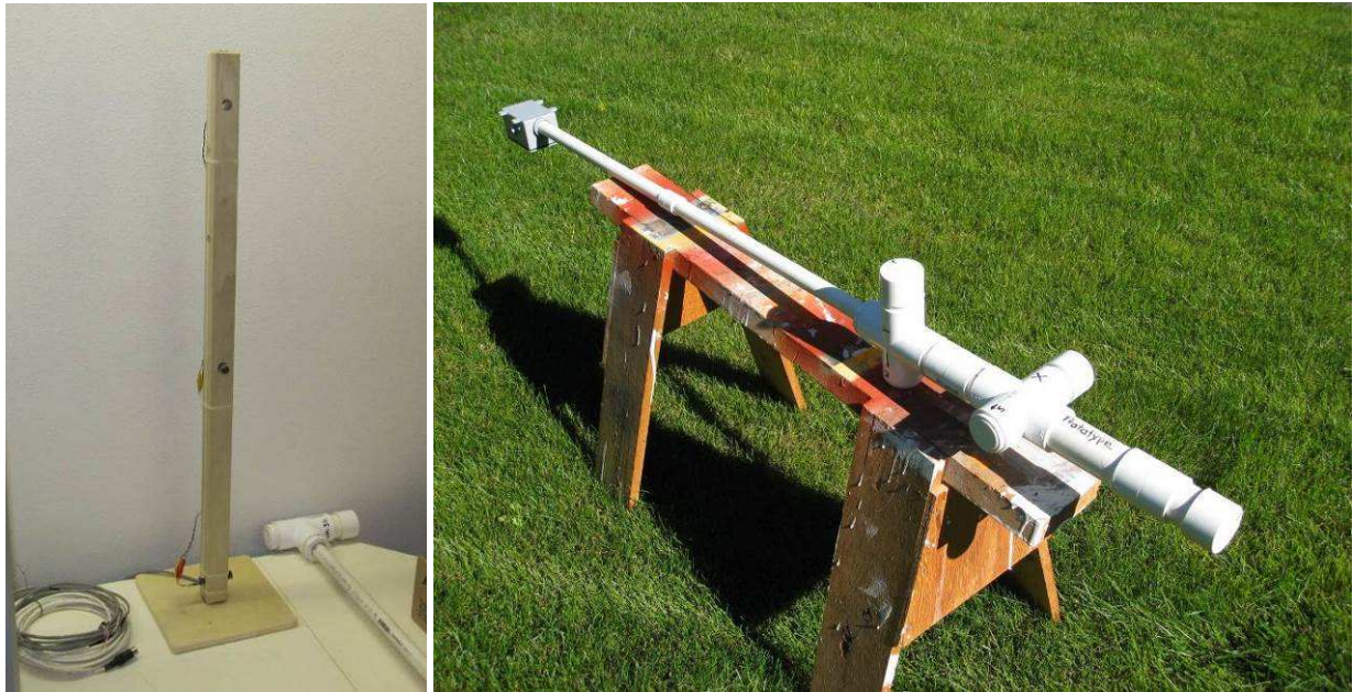
Figure 2 ~ Sensor fixtures. Left : Indoor lab sensor test fixture. The sensors are the small black objects spaced on the vertical wood stick, which is slightly < 1 m long. The X-axis sensor is located at the bottom, Y-axis is 300 mm above X, approximately in the middle, and Z-axis is 300 mm above Y at the top of the stick. The test fixture base is about 0.8 m above the lab baseboard heater and influenced by heat from it. Connections are made by clip-leads. Right : Outdoor sensor fixture posing on a sawhorse before burial in 2010. It was built using plastic DWV pipe and buried vertically so the middle sensor (the first perpendicular cylinder from the right) is about 1 m below the surface. The Z-axis is at the bottom (lower-right corner of the picture), X-axis above it (diagonally to the left in the picture) about 150 mm and Y-axis is closest to the surface and about 150 cm above X. The junction box for connecting the sensor cables is seen at the upper-left corner of the picture.
