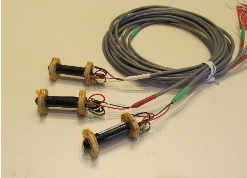
figure 9 ~ Sensors. The sensor pins connect through a pluggable wire mount housing whose terminal contacts have been moisture- and corrosion-protected with dielectric grease. Each sensor was wired to a 3-conductor cable. Wood disks were cut with a hole saw and glued to the sensor to keep it centered when placed in the sensor fixture tubes. The outside diameter of the disks matches the inside diameter of the fixture tubes. The plywood pieces were notched to provide three gaps to allow air convection within the fixture and then coated with epoxy resin. The sensors cabling is color-coded for easy identification. Image © 2022 W. Reeve
