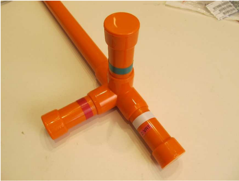
Figure 12 ~ Lower portion of sensor fixture. The sensor fixture for the development system was made from 1 in trade size PVC pipe and a 4-way crossed-tee, the latter providing the correct 90° orientation of each of the three sensors. The sensors, pictured above with wood disks, are held in position with hot-glue. Colored tape, which matched the sensor cables, was used for identification of the sensor tubes. The sensor fixture includes a standpipe (toward upper-left of image) that carries the sensor cabling to the above-ground Remote Interface Junction Box. Image © 2022 W. Reeve
