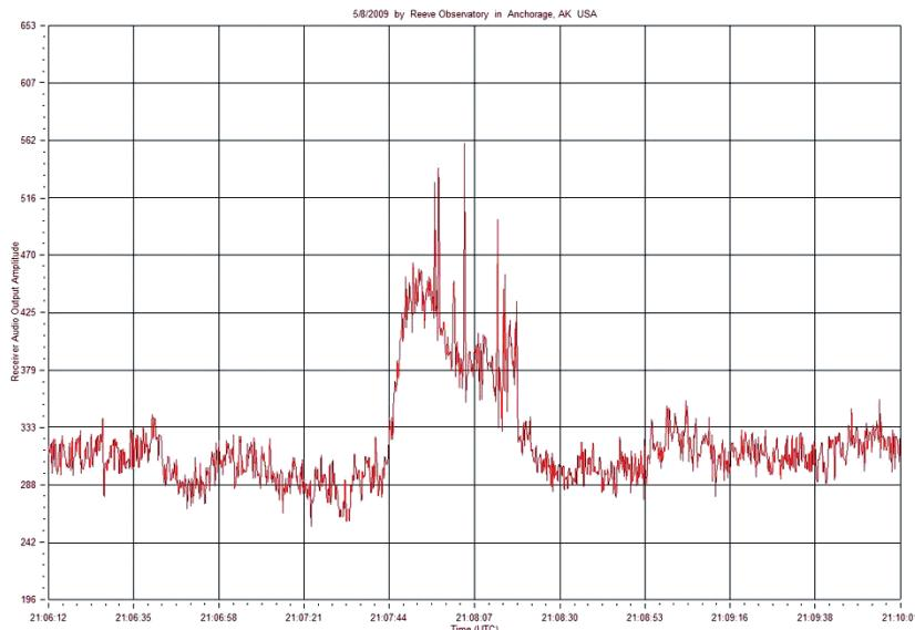
**Fig. 1:** The solar burst is the ‘shark-fin’ shaped event in the centre. The spikes were caused by tuning around the 20.1MHz centre frequency to verify the wideband nature of the burst. There were several stations in the tuning range and each one caused a spike as I tuned through it.
