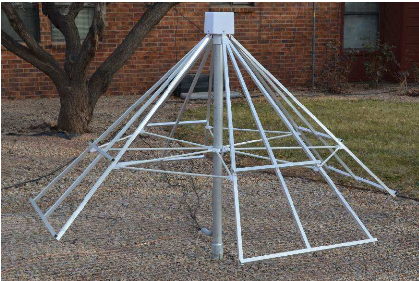
Figure 1-1 ~ Crossed-dipole antenna installed by radio astronomer Stan Nelson at Roswell, New Mexico in January 2014. Each of the two dipoles consists of two triangular aluminum frame elements sloping down 45° and supported from the steel center post by non-conductive horizontal fiberglass rod braces. Each element is 1.5 m long x 0.8 m wide. At the base of the antenna is a 3 m x 3 m galvanized wire mesh ground screen. The peak (apex) of the two dipoles is 1.5 m above ground level with the dual active balun assembly in the gray enclosure at the top. Two coaxial cables can be seen leading away from the antenna, one for each dipole (Image © 2014 S. Nelson, used with permission)
