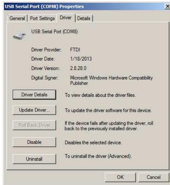
Figure 4 ~ Device Driver Properties – Driver tab for a USB-Serial Adapter
