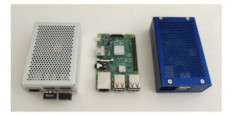
Figure 2 ~ Raspberry Pi model B and B+ hardware. The model B+ is shown in an aluminum enclosure with USB WLAN and BlueTooth dongles (left) and with no enclosure (middle). The model B (right) also is in an aluminum enclosure. The interfaces vary slightly between the model B and B+ but Callisto-Pi works on both models. Enclosure dimensions are approximately 100 x 65 x 25 mm. (Image © 2014 W. Reeve)
