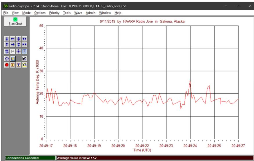
Figure 6 ~ Representative 10 s period starting 2049:17 UTC near the time of minimum background noise level at HAARP. The average of all viewed samples is found by right-clicking the window and selecting *Get Avg for View*. The average value then appears in the lower status bar. For the samples shown here, the value is 17.2, or when scaled is 17 200 K.
