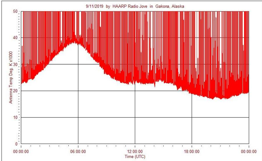
Figure 3.e ~ Averaging bin size = 1000. Compared to figure 2, the baseline amplitude has increased about 2000 K.
