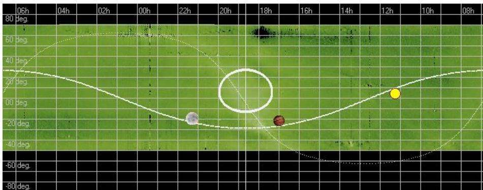
Lower: RadioEyes II plot for HAARP coordinates showing idealized antenna pattern superposed on the 35 MHz radio background. The central meridian is set to 0600 corresponding to the time scale above.
