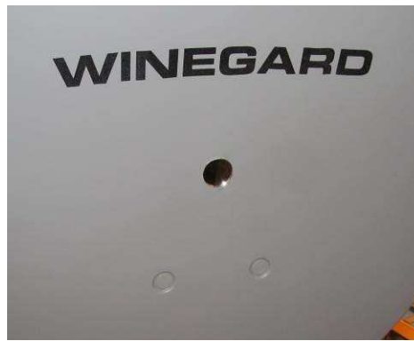
Figure 12 ~ Offset feed dish antenna. Left : Typical offset angles OA are 17 to 24°. Right : One method to align the antenna on a sunny day is to tape a small mirror to the dish center and then adjust the antenna so the Sun's reflection shines on the center of the LNB. A 25 mm diameter mirror from a local craft store is shown in this image attached to the center of a Winegard 46 cm dish.
