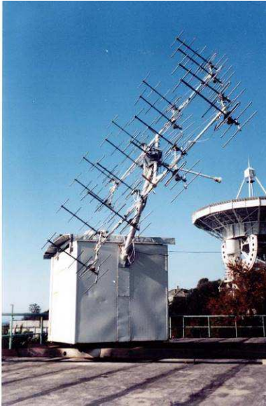
Figure 8 ~ 4 X 4 Yagi array at Radio Astronomy Laboratory of CrAO in Crimea. Each of the sixteen Yagi antennas has six elements. While tracking the Sun, the entire enclosure rotates in azimuth on a vertical axis and the support arm rotates in elevation on a horizontal axis. The estimated gain of each Yagi is 11 dBi and the estimated overall gain of the array is 23 dBi. Image courtesy of C. Monstein.
