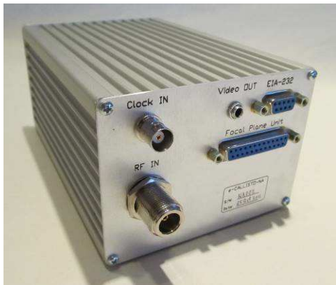
Figure 4 ~ Callisto is a channelized sweep-frequency receiver. In most configurations, the channels are swept at a rate of 800 channels/s, but this can be extended to 1000 channels/s when the Callisto is connected to a 1 MHz reference clock source. The Callisto instrument dimensions are 200 x 110 x 82 mm and it weighs 0.9 kg. It is powered by a 12 Vdc power supply and controlled through an EIA-232 interface. Image ©2012 W. Reeve
