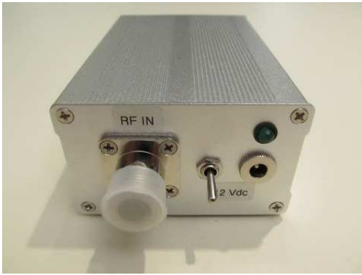
Figure 6 ~ Inexpensive amplifier package made with a modular low noise amplifier. Dimensions are 110 x 77 x 47 mm and average measured noise figure across the frequency range 45 to 870 MHz is 0.8 dB. This unit requires 12 Vdc at 40 mA, and it can be powered through the coaxial cable using a pair of bias-tees or directly with a separate power cable. It is not weatherproof so it must be covered if there is rain during the eclipse. Image ©2015 W. Reeve
