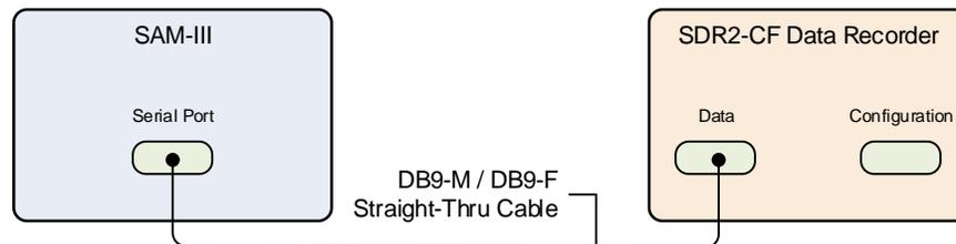
Figure 2 ~ Data connections for deployment (power connections not shown). See also Note in figure 1.
