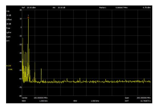
Figure 4.c ~ SatTime output spectra from 0 to 200 MHz before OCXO replacement. The output at frequencies above 10 MHz is clean compared to the subharmonics. The strongest harmonic of 10 MHz is 20 MHz at about –50 dBc.
