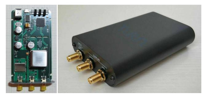
Figure 5.a  $\sim$  Left: System PCB for one of the two units evaluated. The OCXO is the large, square silver can; note the newer appearance than the BG7TBL-D and SatTime (before replacement). The 10 MHz and 1 PPS outputs and antenna input are at the bottom, and the dc power jack, Micro-USB connector and LED indicators are at the top of the image. <u>Right</u>: View of the output and antenna input panel. The outputs are 10 MHz sinewave and 1 PPS.
