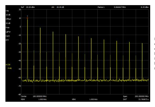
Figure 6.b ~ The MPGPSRC output spectra indicates an offset squarewave with harmonics spaced at 10 MHz intervals. The strongest harmonic is the 3<sup>rd</sup> harmonic (30 MHz) at -10 dBc.
