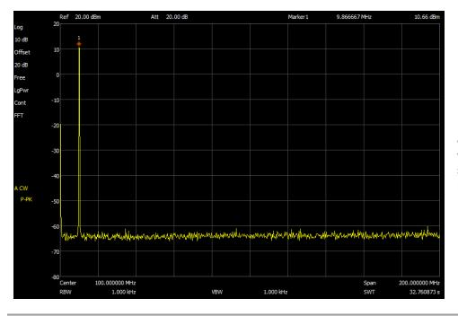
Figure 5.b ~ The TM4313 output spectra is very clean with no visible spurious signals or harmonics with a power level above –75 dBc.
