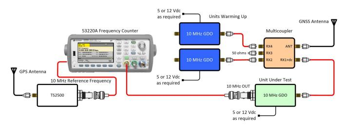
Figure 2 ~ Block diagram of measurement setup. The Unit Under Test (UUT) provides powering voltage to the active GNSS antenna while the other units are warming up and tracking for at least 24 hours. The GDOs were rotated through so that all eventually powered the GNSS antenna as part of the evaluation. Because the frequency counter and UUT used separate receivers and antennas, they operated plesiochronously.
