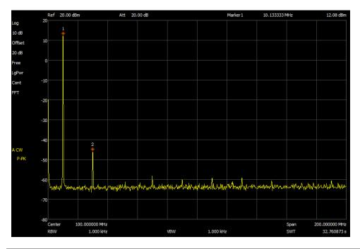
Figure 7.b ~ The PLL-GNSSDO output spectra is very clean with only the fundamental and  $3^{nd}$  harmonic (30 MHz) visible. The  $3^{nd}$  harmonic level is -58 dBc.
