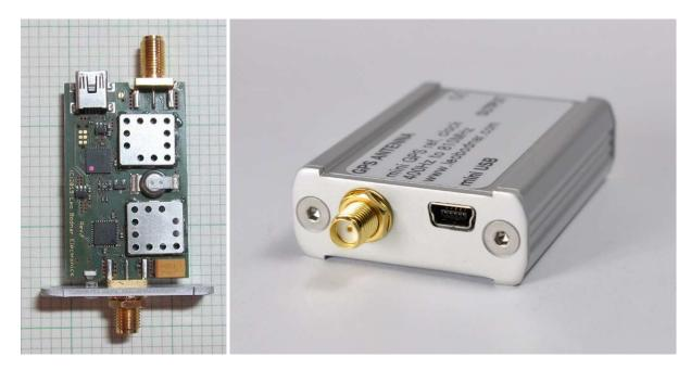
Figure 6.a  $\sim$  Left: System PCB. The TCXO is presumably under one of the metal shields. The output is at the bottom and the antenna input and Mini-USB connector are at the top of the image. The only output is a variable frequency squarewave the frequency of which is set by the user; I set my unit to 10 MHz; <u>Right</u>: View of the antenna input and Mini-USB connector panel. Image source: leobodnar.com
