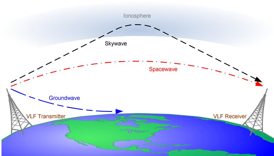
Figure 2 ~ Propagation at VLF and LF consists mainly of groundwaves and spacewaves. The groundwaves dissipate over relatively short distances, but the spacewaves use an Earth-Ionosphere waveguide mode that supports propagation over thousands of km. The skywave is important at higher frequencies but generally not used by VLF and LF radio waves. Image ©2010 W. Reeve.
