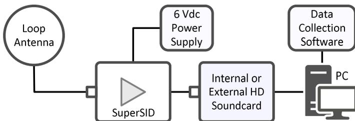
Figure 4 ~ Block diagram showing the SuperSID VLF monitor. The SuperSID includes a 6 Vdc power adapter and necessary software. It works best with a high definition (HD) internal or external soundcard that supports at least 96 kHz sampling rate, in which case the SuperSID can monitor a range of frequencies up to about 48 kHz. Image ©2016 W. Reeve.
