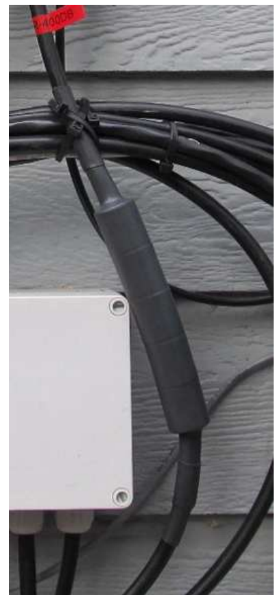
Figure 4 (right) ~ A choke balun is made by slipping several ferrite beads over a coaxial cable. This image shows five solid beads on LMR-400 cable that have been covered with heatshrink tubing.
