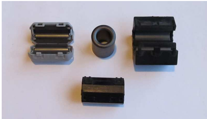
Figure 1 ~ Ferrite beads used for noise suppression. A solid bead (upper-middle) is shown surrounded by clamshell beads. The clamshell bead is split into two identical pieces and held together by a plastic housing with clasps. The mating surfaces of the clamshell bead are very smooth so that when they are clamped together there is negligible air gap. Ferrite beads are available in many lengths and inside and outside dimensions and different material mixes. Beads with a rectangular slot are available for flat cables.
